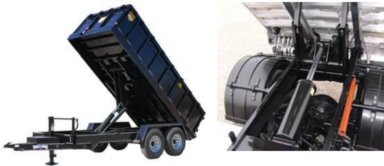
Underbody application on small dump trailers
