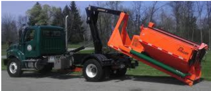
Swap-loader Hook Lift Systems using Custom Hoist Hydraulic Cylinders
