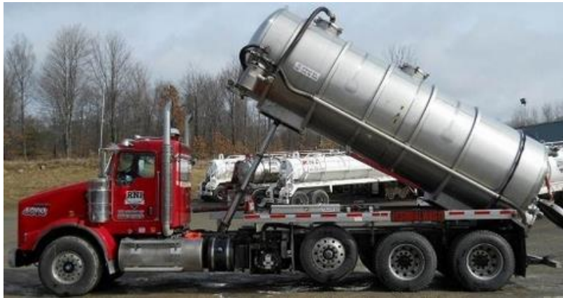
Liquid Refuse with Double Acting Telescopic Cylinder
