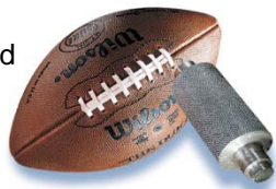
Engraved rolls used for producing surface textures on everyday items
