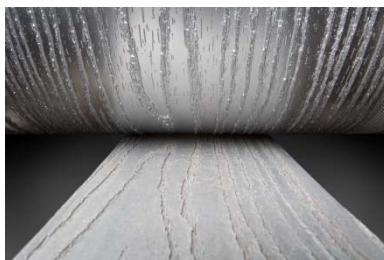
Engraved rolls used for producing surface textures on everyday items
